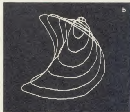
Figure 1. Lofting to input 3D data: a) object defined as a set of height contours; b) object as a 3D solid
